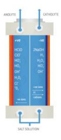
Anolyte Water, a mixed oxidant, is produced by electrolyzing dilute brine(NACL) water in the cathode & anode chamber of an unique diaphragmatic electrolytic cell. An electro-chemical activation is used to convert an aqueous solution of sodium chloride into a solution known as "Anolyte."
